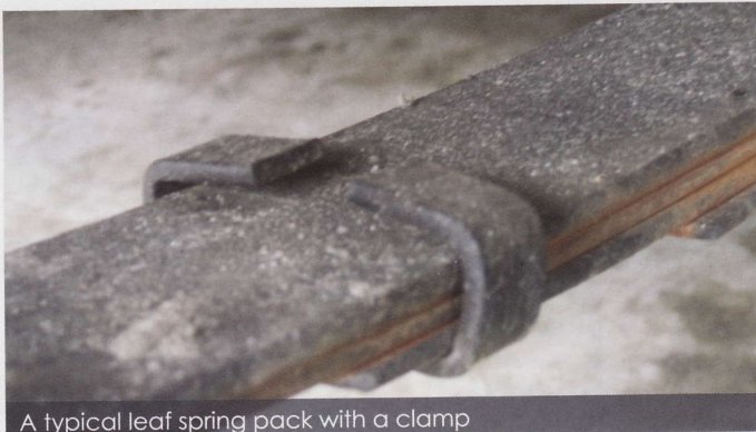
A typical leaf spring pack with a clamp
