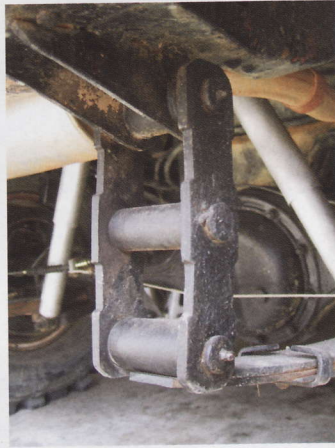
Longer shackles are popular among offroaders - a simple way of increasing ride height
