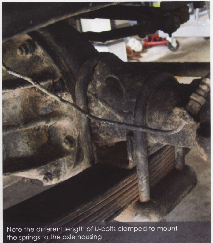
The forward mounting of the spring is fixed, while the rearward is shackled connected
