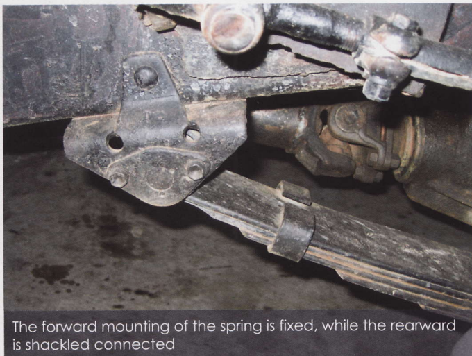
Note the different length of U-bolts clamped to mount the springs to the axle housing
